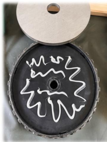
After applying the adhesive, the discs can be inserted into the wheel. Please make sure to insert them as centrally as possible, towards the rim hole.
